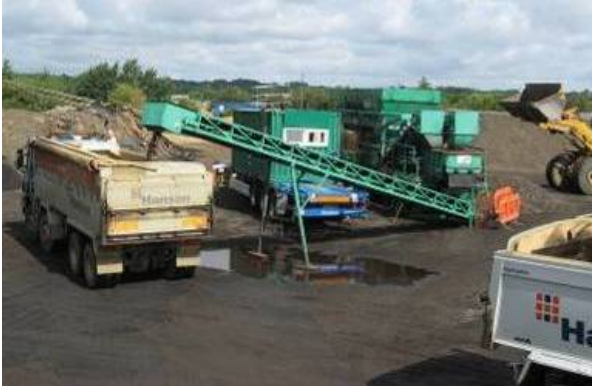
Cold emulsion asphalt manufacture with recycled aggregate
