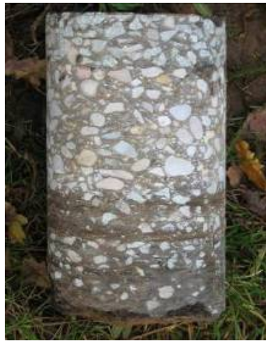
Cold emulsion structural asphalt installation and core specimen.
