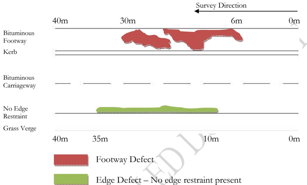
**Figure 1 CVI Length Defect**
