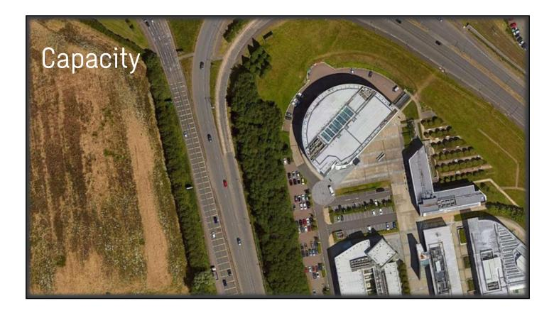
The southbound carriageway has just come off a roundabout with three lanes, which narrows to two lanes just at the point where a dedicated left turn from the previous roundabout arm merges. Effectively providing a four to two lane merge.
