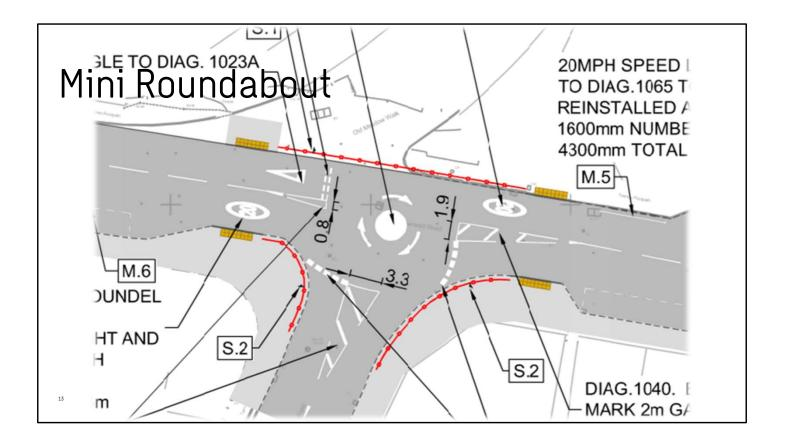
Mini roundabouts require users to drive around the central island – it can be overrun if the vehicle you are driving is too big though.
