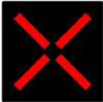
Red-Cross (lane control) aspect TSRGD Diagram 5003.1
