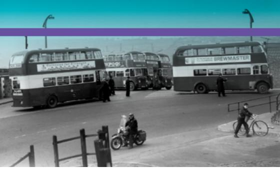
The buses themselves were mainly the traditional half cab double deckers with the engine at the front, an open rear platform and staircase usually seating 56 people in a very compact 27ft by 7ft 6ins (approx 8m by 2.25m) with a crew of two, a driver and conductor.
