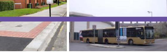
In more recent years the requirements of the Disability Discrimination Act (DDA) along with parallel EU directives have led to the widespread introduction of low floor buses. In order to take full advantage of these, kerbs have been raised at bus stops and in places specially designed kerbs such as the Kassel Kerb have been used to enable the bus to get as close to the stop as possible without damaging the tyres.
