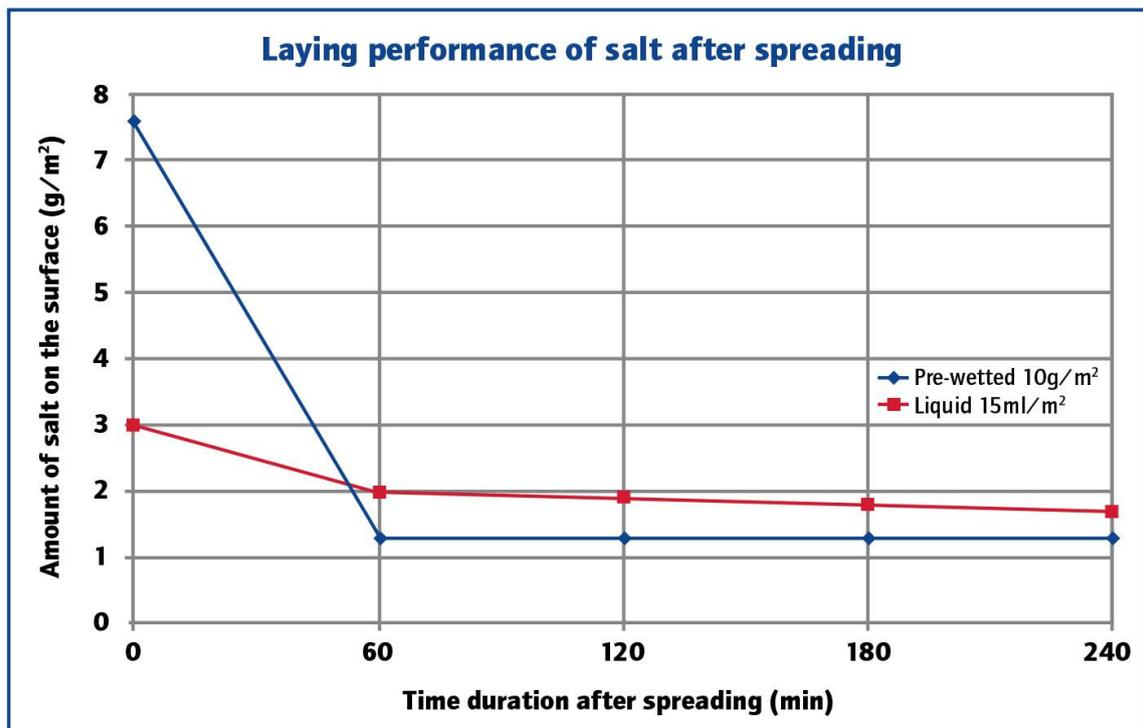
Figure 1: A comparison between pre-wetted and liquid spreading for winter pre-treatments
