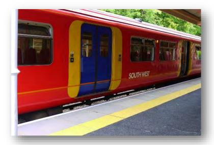
Platform edge (off-street) warning surface – used at railway stations to indicate you are close to the edge of the platform.
